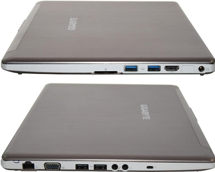
Connectivity-wise, you'll find an SD card reader, two USB 3.0 ports, HDMI port and a DC-input power jack on the right side. The left side includes a Gigabit Ethernet port, D-sub (VGA) port, two USB 2.0 ports, microphone jack, headphone jack and a Kensington lock slot.
