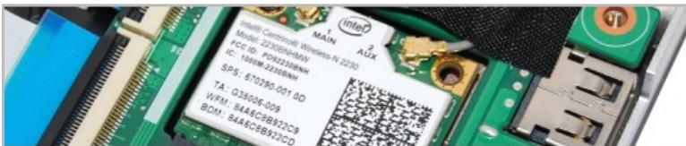
The U2442F's internals are dominated by the motherboard, a green PCB measuring 260mm by 140mm. The vast majority of the [hardware](#) components are on this PCB, though there is a smaller 60mm by 140mm PCB on the right side which houses the Wi-Fi and Bluetooth card along with a few USB ports.
