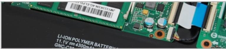
At the front of the [Ultrabook](#) is the Li-polymer (11.1V, 47.73Wh) battery which measures 210mm by 75mm and is just 10mm thick. Adjacent from the battery is a 2.5" hard drive. Our review unit came with the Toshiba MQ01ABD075, which is a 750GB, 5400-RPM, SATA II drive.
