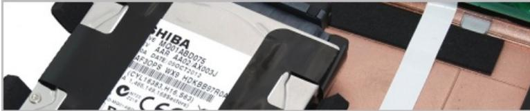
Interestingly, the 2.5" hard drive is not screwed into the Ultrabook but rather it just sits in place inside a rubberized caddy which not only holds the drive but also reduces vibration and therefore noise.
