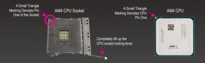
Once the CPU is positioned into its socket, place one finger down on the middle of the CPU, lowering the locking lever and latching it into the fully locked position.
