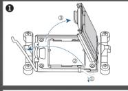
Hold the CPU with your fingers by the edges. Align the CPU pin one marking (triangle) with the pin one corner of the CPU socket (or you may align the CPU notches with the socket alignment keys) and gently insert the CPU into position.
