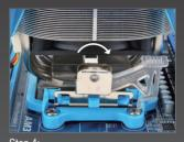
Step 4: Turn the cam handle from the left side to the right side to lock into place. (Refer to your APU cooler installation manual for instructions on installing the cooler.)
