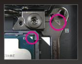
Step 4: Hold the CPU with your thumb and index fingers. Align the CPU pin one mark (triangle) with the triangle mark on metal socket frame and carefully insert the CPU into the socket vertically.
