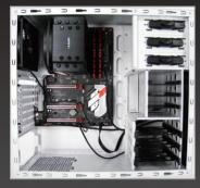
Remove the original I/O shield from the back of the case and replace it with the motherboard I/O shield. Place the motherboard within the case by positioning it into its I/O shield. Align the mounting screw holes on the motherboard with their corresponding mounting holes on the case. Secure the motherboard in place with screws.
