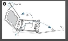
Hold the CPU with your fingers by the edges. Align the CPU pin one marking (triangle) with the pin one corner of the CPU socket (or you may align the CPU notches with the socket alignment keys) and gently insert the CPU into position.
