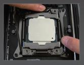
Step 5: Once the CPU is properly inserted, carefully replace the load plate. Then secure lever B under its retention tab
