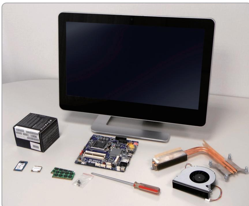
Note: The CPU heatsink and fan are supplied with the chassis and are specific to that chassis design. Some chassis manufacturers may specify certain limitations regarding CPU model compatibility due to thermal design constraints.
