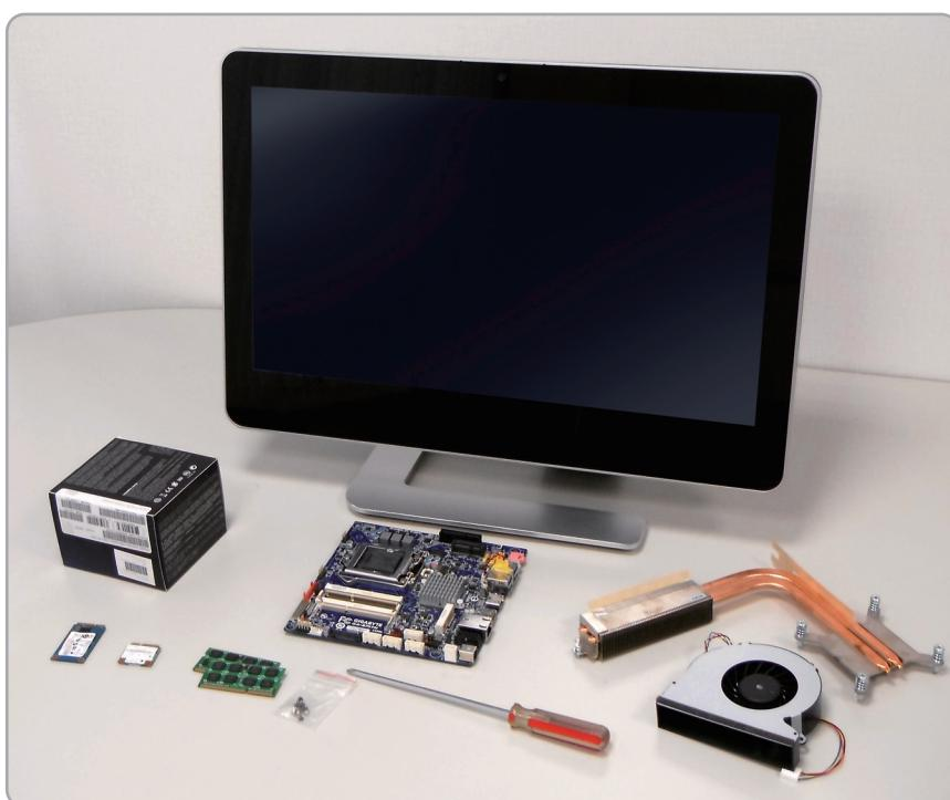
Note: The CPU heatsink and fan are supplied with the chassis and are specific to that chassis design. Some chassis manufacturers may specify certain limitations regarding CPU model compatibility due to thermal design constraints.
