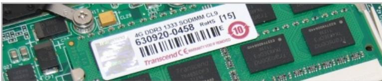
Both DIMM slots are loaded with a pair of DDR3-1333 4GB sticks for a total capacity of 8GB. The 3rd Generation Intel Core i7 [processor](#) consists of the i7-3517U (1.9GHz - 3.0GHz), though it is also possible to get the slightly faster i7-3537U (2.0GHz - 3.1GHz) processor in this same model.
