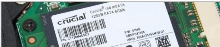
Along the 750GB 2.5" hard drive there's a mSATA slot which can be fitted with either a 128GB or 256GB SSD. Gigabyte has picked the highly regarded [Crucial m4](#) which is a high speed SATA 6Gb/s SSD.
