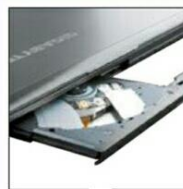
The P35X V3 comes with a DVD-RW optical drive, although you can swap it out for a Blu-ray drive or an extra HDD.
